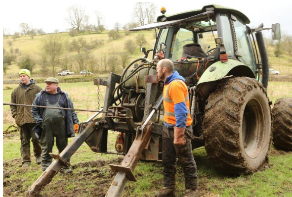
Fig. 1: Tractor winch used in tree winching
